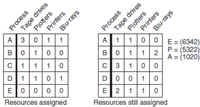
Figure 4.5 The banker's algorithm with multiple resources (Reference: "Modern Operating Systems" by Andrew S Tanenbaum)
