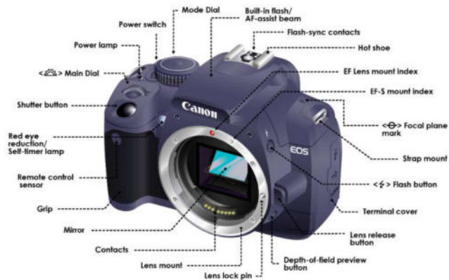
Parts of DSLR
