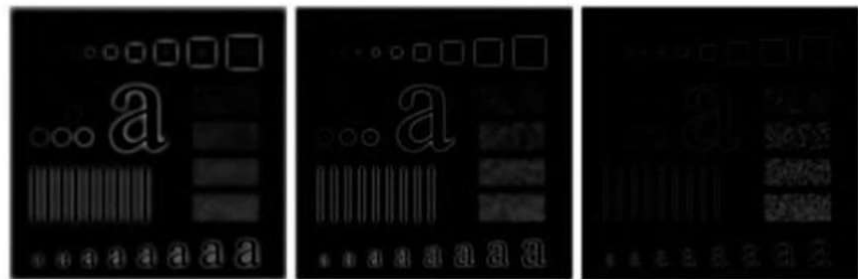
Figure 15: Results of highpass filtering the image using a BHPF of order 2 with D_0 = 30, 60 and 160
