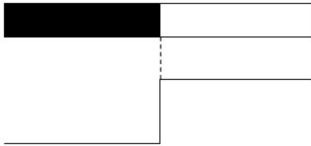
Figure 2. A step edge and their corresponding intensity profiles
